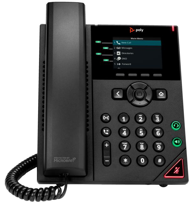
POLY VVX 250 4-Line IP Phone and PoE-enabled. Product type: IP Phone, Product colour: Black, Handset type: Wired handset. Lines quantity: 4 lines. Display: LED, Display diagonal: 7.11 cm (2.8"), Display resolution: 320 x 240 pixels. Voice codecs: G.711, G.722, G.722.1, G.729ab, OPUS, iLBC. Ethernet LAN interface type: Gigabit Ethernet, Ethernet LAN data rates: 10,100,1000 Mbit/s, Security ...
